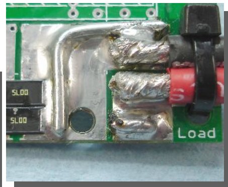
Fig.3 Wire from Sense Resistors to Load
